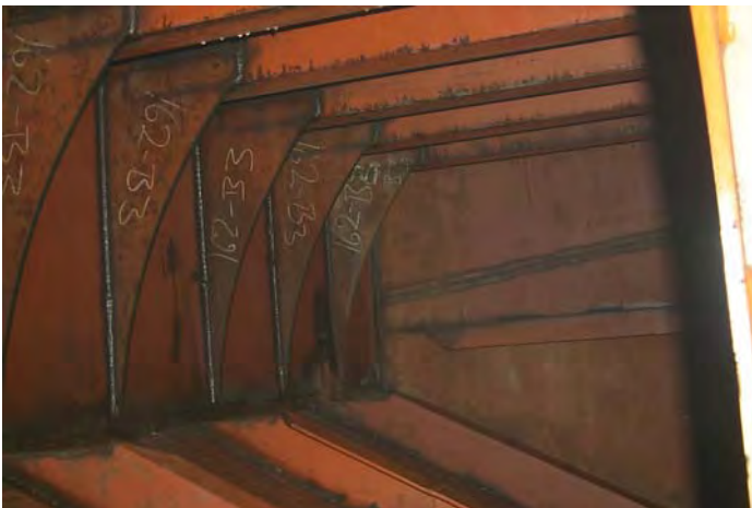
Internal structure of a 30 m 10-year-old barge.
